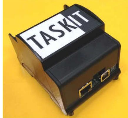
Built with a standard TaskIT controller TS87J60-ETH-USB, integrated with a specific Analog Front End daughter board.
